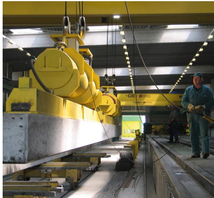
Precast concrete elements are factory made under strict controls. The manufacture of structural elements is automated to a considerable extent. Courtesy of British Precast and Bond van Fabrikanten van Betonproducten in Nederland (BFBN).
